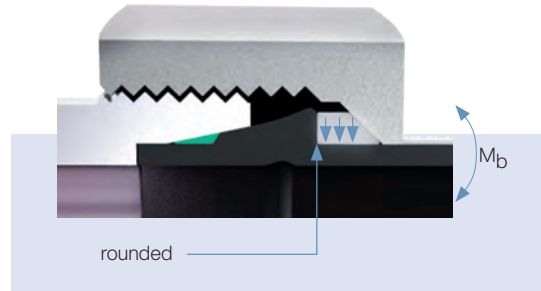
Dynamic load absorption by integrated clamping ring
