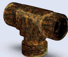
Zinc + passivation + sealing coat
