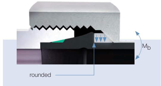
Dynamic load absorption by integrated clamping ring
